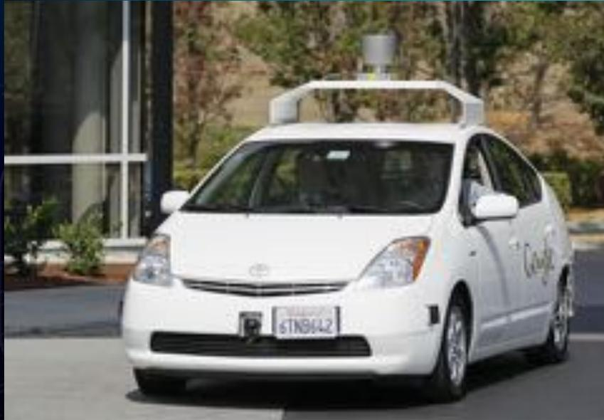
LiDAR uses light to measure the distance from a sensor to an object. A light beam is scanned over an area and an accurate 3d map generated using the reflected time data.
